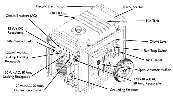
**12 Volt DC Receptacle** — Use this receptacle with battery charge cables to charge a 12 Volt battery.
